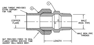
PARTS AND MATERIAL: 1. BODY: CAST BRASS, ALLOY C89833 2. NUT: CAST BRASS, ALLOY C83600
