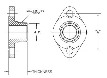
PARTS AND MATERIAL: FLANGE: CAST BRASS, ALLOY C89833 BOLT: STAINLESS STEEL, 304 NUT: STAINLESS STEEL, 304 GASKET: NEOPRENE
