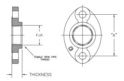
PARTS AND MATERIAL: FLANCE: CAST BRASS, ALLOY C89833 BOLT: STAINLESS STEEL, 304 NUT: STAINLESS STEEL, 304 GASKET: NEOPRENE
